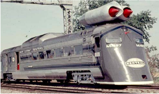
New York Central modified Budd RDC-3 with jet engine pod.
