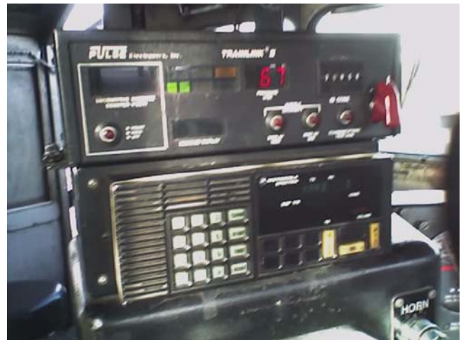
A typical "Wilma," or Head-of-Train Device (top unit), displaying the current brake pipe pressure on the rear end.
