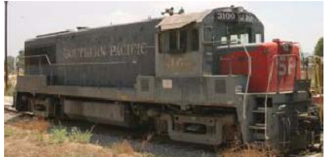
This GE U25B No. 3100 is believed to be the only remaining operable locomotive of its type in the U.S.
