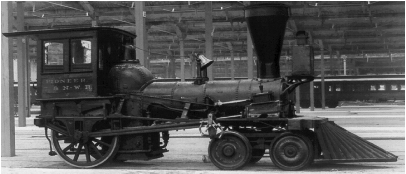
The Pioneer as it appeared in 1883. The boiler jacket, large whistle, and tender have disappeared.
