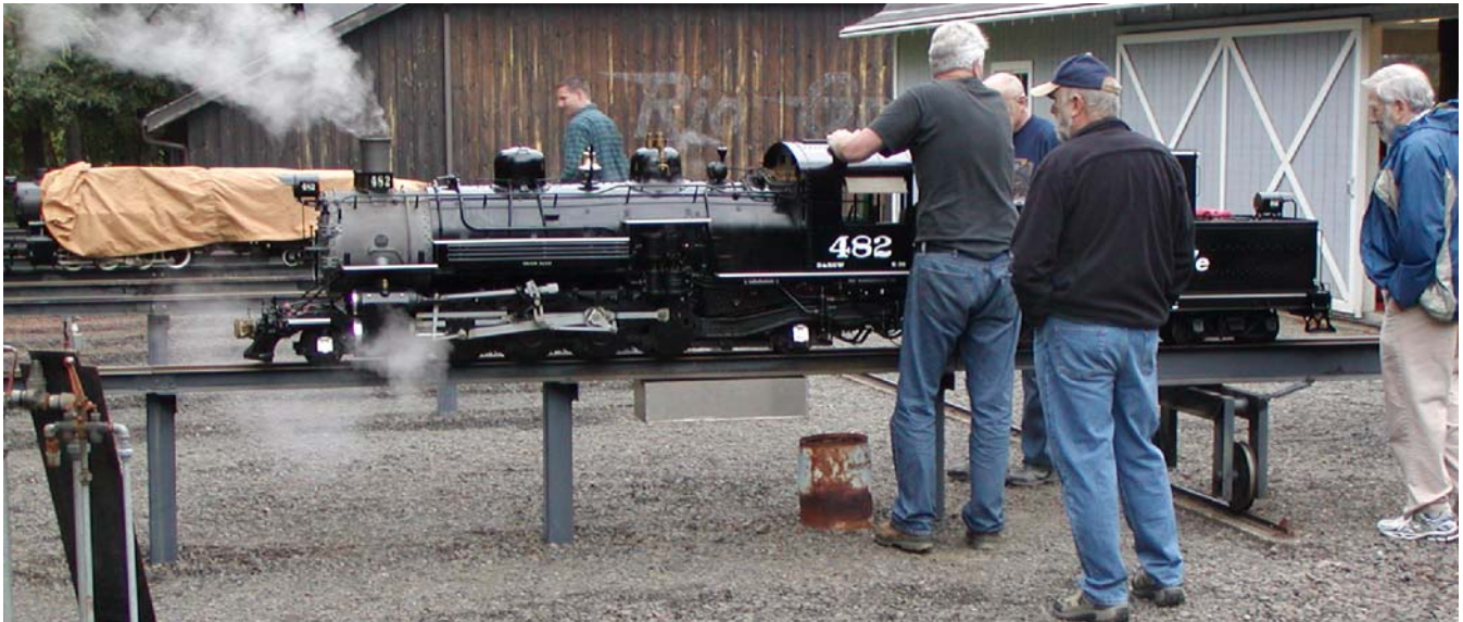
Dumping the fire into the ash pit. Notice the thermal blanket on the other locomotive.
