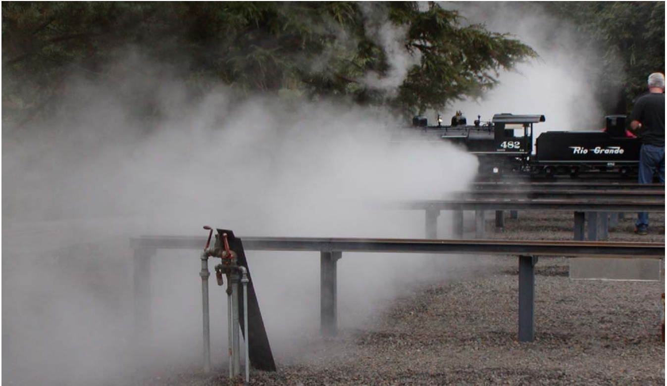
Boiler blow down to release the steam pressure.
