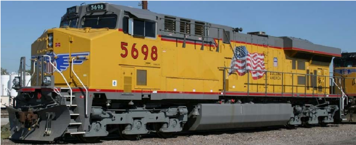
GE C45AC-CTE Evolution Locomotive with the GEVO 12-cylinder diesel engine
